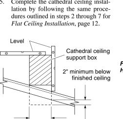
Cut hole 1/8" larger than support box when projected onto roofline
